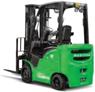
Electric Lithium-ion Cushion Tire Forklifts 3,000-15,500lbs
