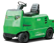
Electric Lithium-ion Tow Tractors 4,500-70,000lbs
