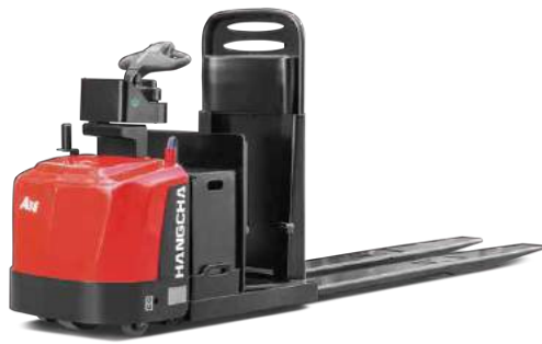
A Series Walkie Counterbalanced Stacker Capacity 2,000~4,000lbs
